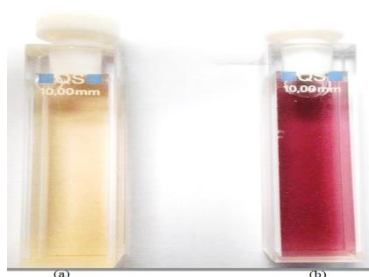
Figure 2. The color of a) Fe(III)-EDTA- \text{NH}_3 and b) Fe(III)-EDTA- \text{NH}_3 - \text{H}_2\text{O}_2 complex.
